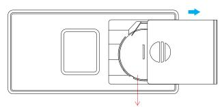
Note:Before the first use, please remove the protective film on the battery.
