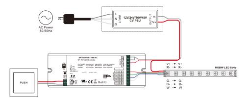
Note: please make sure the dial switches are at position for RGBW mode as shown in above diagram.
